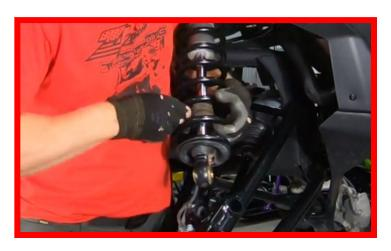
Now slide the spring stack down to completely remove it from the shock body.
