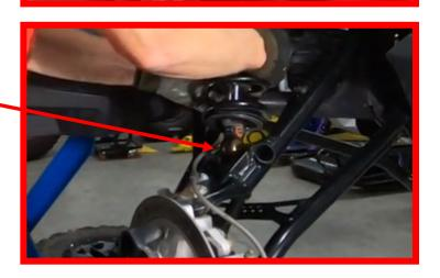
Take a measurement from the top of the Crossover Nut down to the Top of the Main Spring. This should be 4.25" to begin with. \*Additional Preload may be needed depending on after-market accessories (bumper, cage, tire carrier, stereo system). You can put more pre-load on by repeating turning the pre-load nut more.
