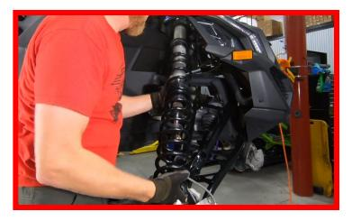
Take the OEM Main Spring and Spring Divider and place the new ZBROZ Tender Spring on Top. Slide the Spring Stack back up through the shock body.
