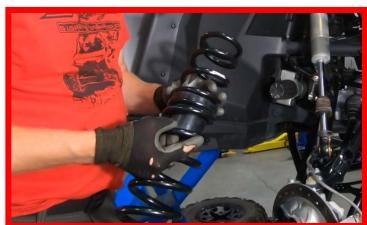
Next Place the lower Spring Retainer back on the same way it came off and then mount your shock back to the A-Arm with the lower shock bolt. Tightening the nut and bolt to factory torque specs.
