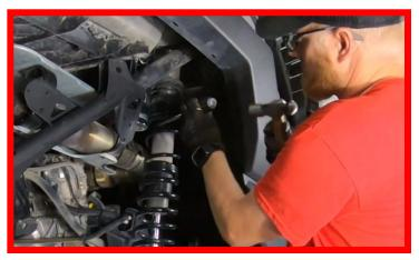
Remove the bottom retainer by lifting up on the spring stack with the help of another person or by using a Strut Compressor tool. This is the same process as done of the front.
