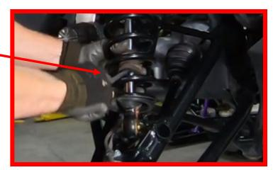
Next, loosen your pre-load all the way up until the collar is all the way to the top. You need to use a hammer and flathead screwdriver to loosen the nut.
