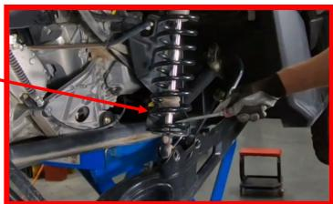
Next, loosen your pre-load all the way up until the collar is all the way to the top, or spring pack is loose.
