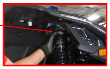
Take a measurement from the top of the Crossover Nut down to the Top of the Main Spring. This should be about 2". If it needs adjustment, you will do this by continuing to rotate the pre-load nut clockwise until your measurement is 2"
